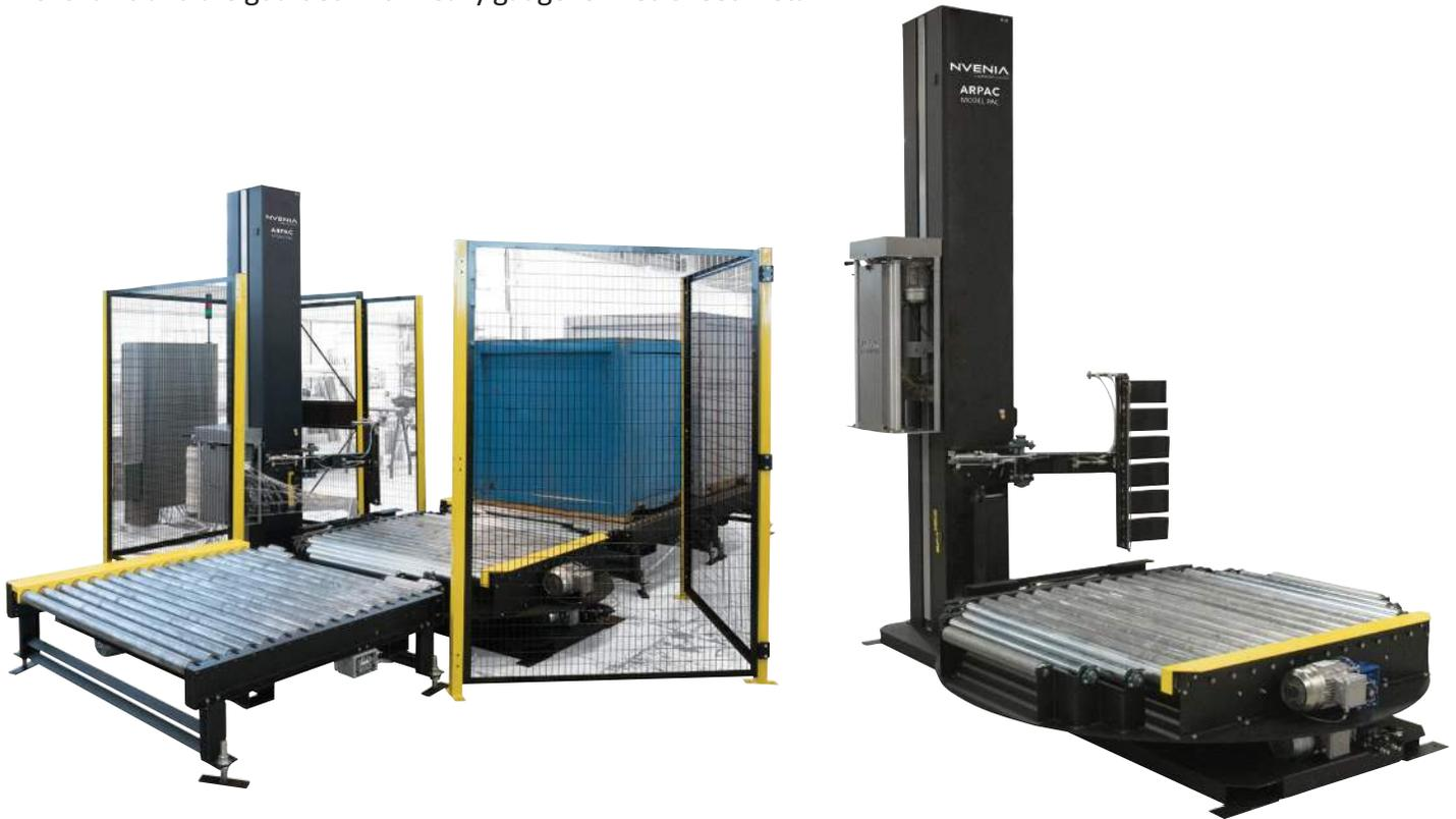
The PAC Model can be manufactured with several performance enhancements. The Roping device is used as a replacement for belly straps and stabilizes the load, and a Top Sheet Dispenser covers the top of the pallet with film, for additional product protection from the elements.
