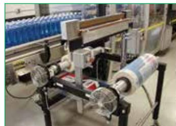
Side Film Rack with Splice Bar
