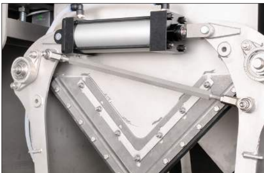
Stainless steel gravity gate and weigh bucket, with hydraulic hinge.
